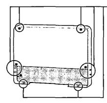
Use these M4 screw holes to mount the LCD Monitor.
